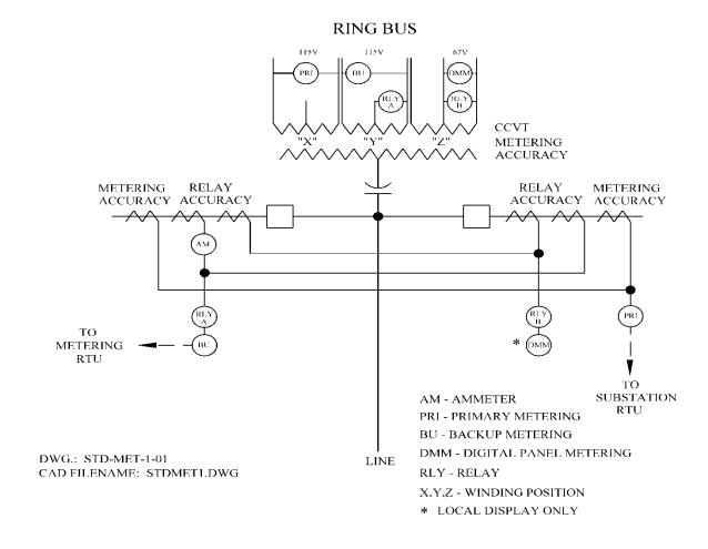
Figure 1. Primary & Backup Interconnection Metering Diagram for Ring Bus
