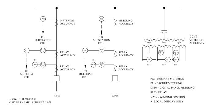
Figure 2. Primary & Backup Interconnection Metering Diagram for Radial Bus
